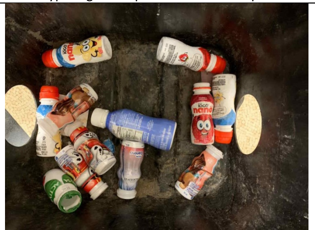
Typical HDPE in sample
